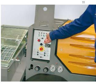
You can control the complete machine from the convenient control panel. A practical flap protects the control panel against dirt and . damage.
