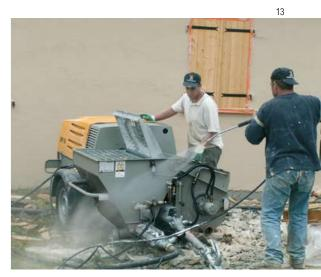
Once your work is finished, you can clean your Beliso with the integrated 120 bar high-pressure cleaner - quickly and efficient.
