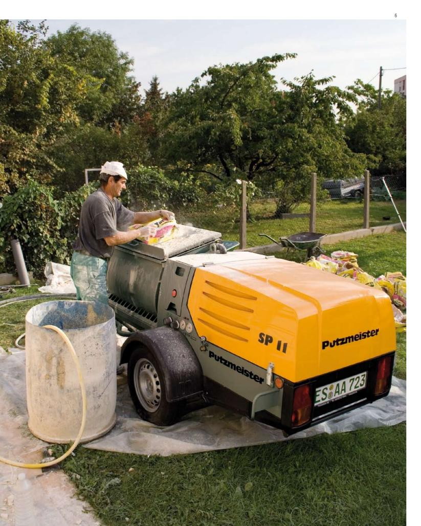
The **trap mixer** (SP 11<sup>BMT</sup>) is the simple, robust and cost-effective variant. This mixer is fixed to the machine. The prepared material flows through a flap in the bottom of the mixer into the hopper of the SP 11.
