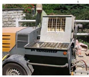
But it gets even better. BMR models have a lifting mixer, on which a powerful hydraulic system does all the work.
