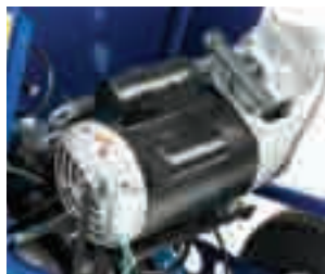
Single motor operates both the pump and the compressor.
